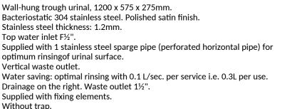
Without trap. Possible to add one or more bacteriostatic 304 stainless steel dividers (ref. 100900). Fix directly onto the urinal in the desired location. Installation advice: if you wish to install 2 urinals side by side, we recommend ordering one urinal with drainage on the left and one with drainage on the right.
