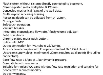
This model does not have a waterproof recessing housing. The installer must ensure that the recessing area is waterproof and any leaks or condensation can drain away (see installation guide).
